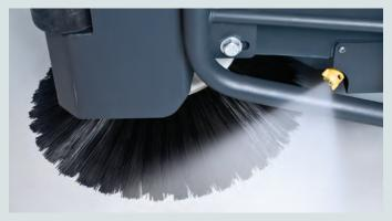
Patented DustGuard™ is proven to reduce airborne dust generated by side broom sweeping. An ultra fine fog suppresses fugitive dust
