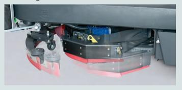
Retractable 10 cm offset disc deck enhances edge scrubbing and resists damage from accidental impact
