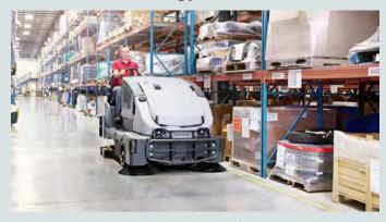
The CS7010 delivers unparalleled performance, while replacing power-hungry, high-maintenance hydraulic systems with efficient, state-of-the-art Electric Drive technology
